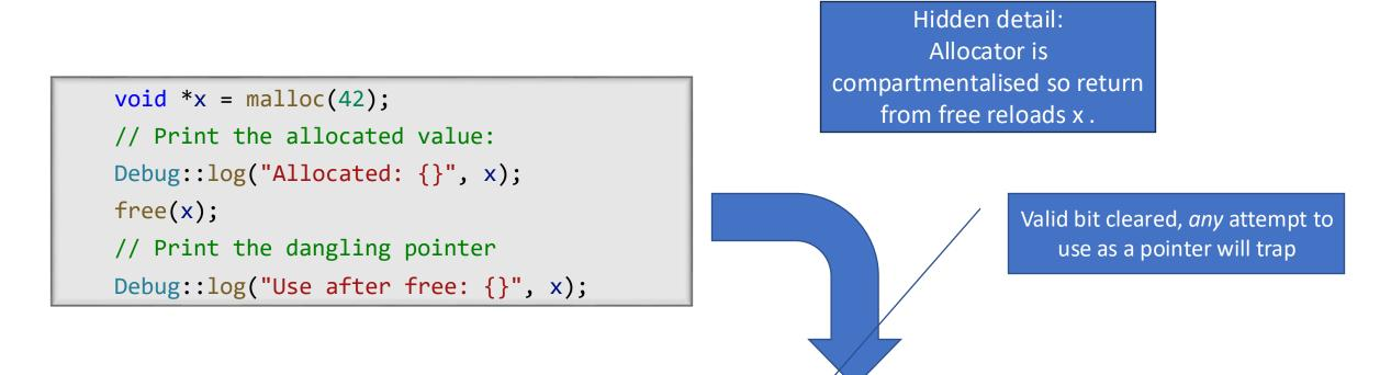
Allocating compartment: Allocated: 0x80005900 (v:1 0x80005900-0x80005930 I:0x30 o:0x0 p: G RWcgm- -- ---) Allocating compartment: Use after free: 0x80005900 (v:0 0x80005900-0x80005930 I:0x30 o:0x0 p: G RWcgm- -- ---)
